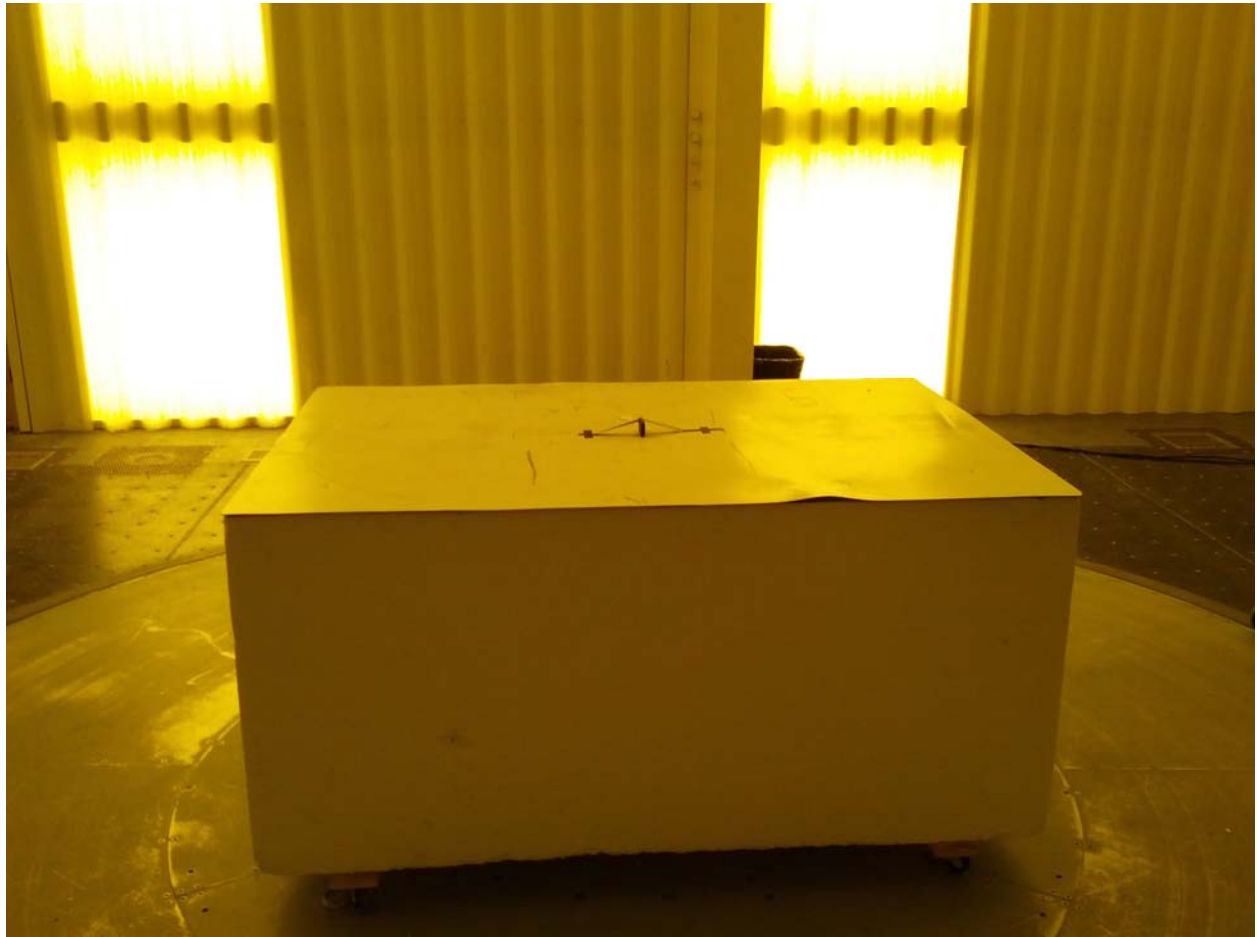
Photograph 1 – Front View Radiated Disturbance Worst Case Configuration (EUT on edge)
