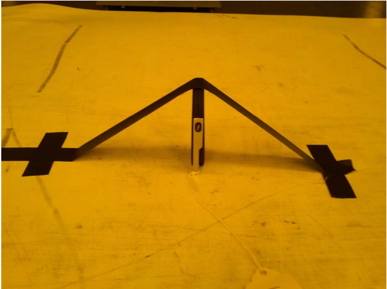
Photograph 4 – EUT Orientation for Radiated Tests - Vertical
