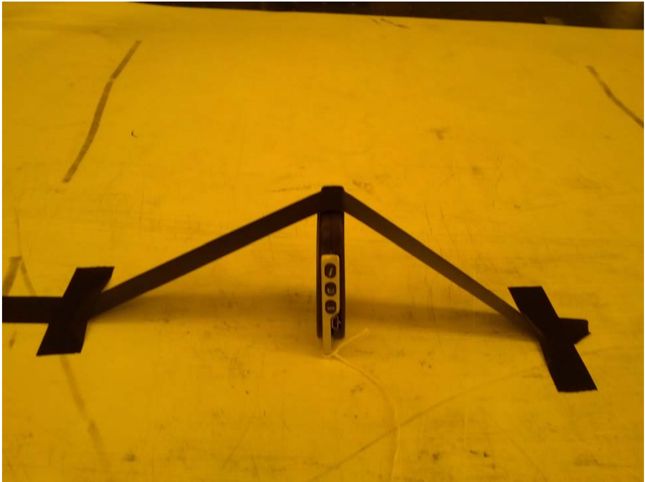
Photograph 4 – EUT Orientation for Radiated Tests - Vertical
