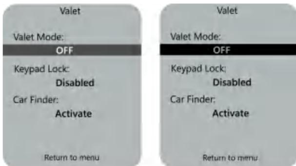
With the feature selected, LOCK and UNLOCK will cycle through the available options for that feature (Valet/OFF).
