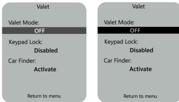
With the feature selected, **LOCK** and **UNLOCK** will cycle through the available options for that feature (Security Valet/Start Valet/Combo Valet/OFF).
