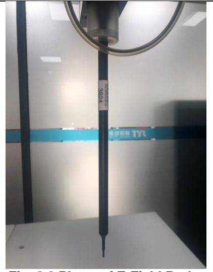
Fig. 8.2 Photo of E-Field Probe
