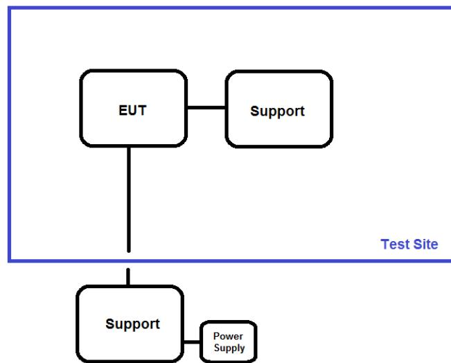
Radiated test setup
