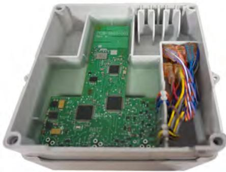
4. To wire the 500W ERT remote module to the RTR 2-wire register, connect the remote 500W ERT module wires to the 2-wire register using gel-cap connectors. After the wires are connected, carefully tuck the connectors into the remote 500W ERT module housing.
