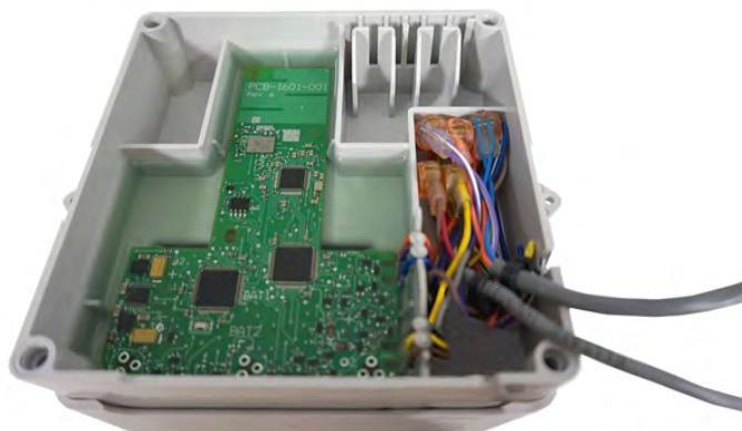
2. Route the register cable through the bottom backplate cable cutout and telemetry device cable through the top backplate cable cutout.
