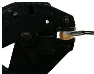
4. A connector is crimped properly when the top of the movable yellow center (1) is flush with the top of the connector body (2).
