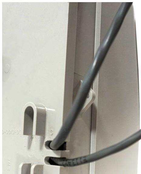
3. Align the remote module backplate with the mounting screw holes. Verify that the Itron logo is not upside down.
