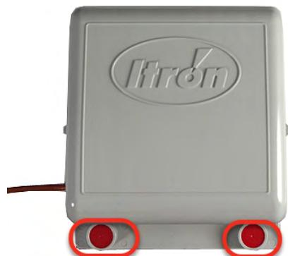
**Note:** A tamper seal is fully seated when the top of the tamper seal is approximately 1/16 inch below the top of the screw recess.
