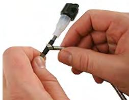
**Important:** You must twist—not wrap—the cable armor onto the pit module cable. Wrapping the cable armor can cause the stainless steel jacket to warp. You must begin twisting the cable armor over portion of the cable protected by the electrical tape. If you do not begin to twist the cable armor over the protected portion of the pit module cable, a cut cable could cause an pit module/register communication failure.
