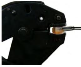
4. A connector is crimped properly when the top of the movable yellow center (1) is flush with the top of the connector body (2).
