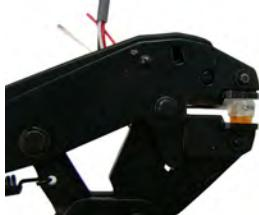
3. Crimp the connector by squeezing the handles until the connector cap is fully seated. Continue to apply pressure for three seconds.
