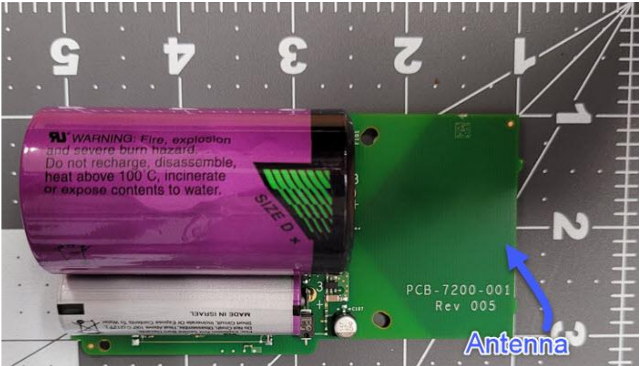
Figure 2: Batteries attach and antenna location
