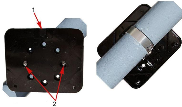
If the pipe is at a 45 degrees angle up to the left, install the adapter plate as shown in the pictures below.
