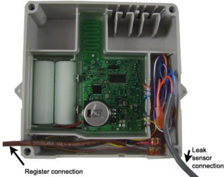
2. Route the register cable through the appropriate backplate cutout and the Leak Sensor cable through the remaining cutout.
