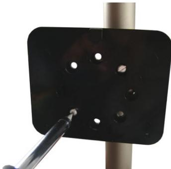
8. Tighten both screws to 9 to 12 inch-pounds of torque.
