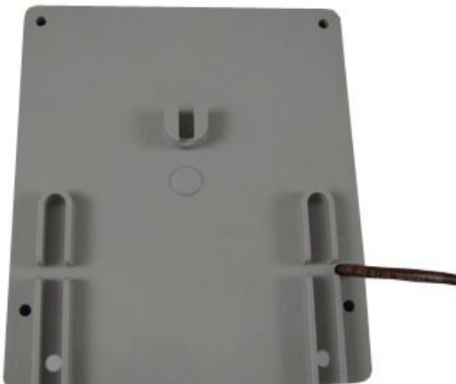
3. Align the endpoint backplate with the mounting screw holes. Verify the Itron logo and arrow point up.
