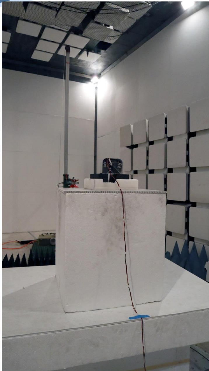
Spurious Emissions ERG-5600-008, 1-18GHz Front, Power Cable Up
