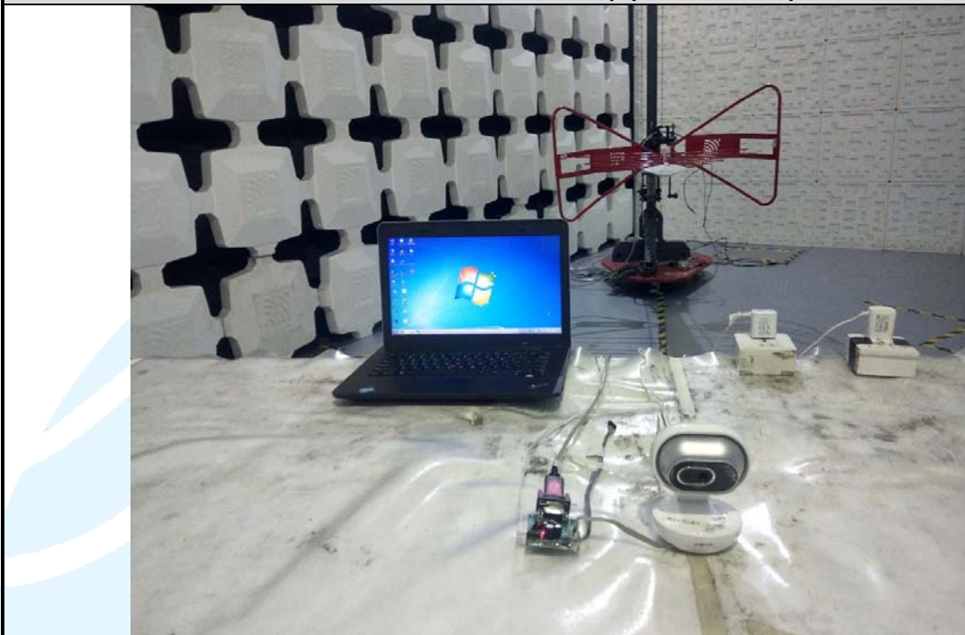
Radiated emission Test Setup (30 MHz~1 GHz)
