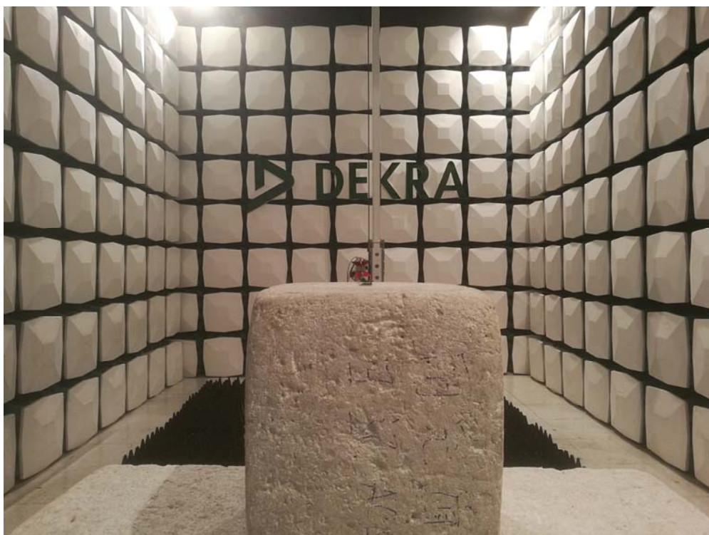
Description: Radiated Emission Test Setup for 1~18GHz
