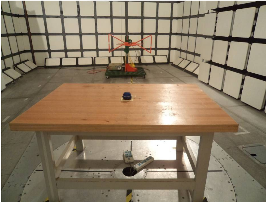
Radiated Emissions View (30-1000 MHz)
