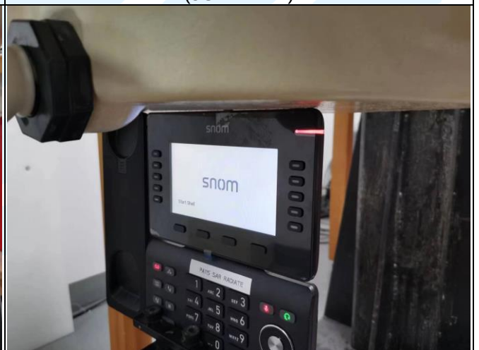
Top Side of EUT with 0 cm Gap (5GHz Wi-Fi)
