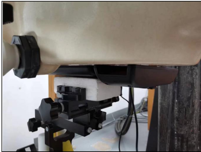
Front Face of EUT with 0 cm Gap (2.4GHz Wi-Fi)
