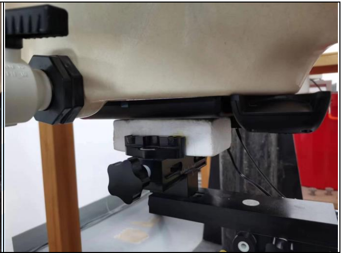
Front Face of EUT with 0 cm Gap (5GHz Wi-Fi)
