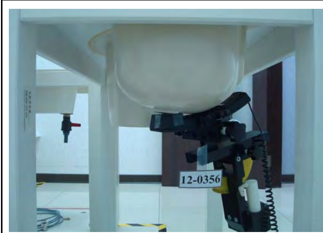
Figure 2. Right Head SAR Test Setup (Cheek)
