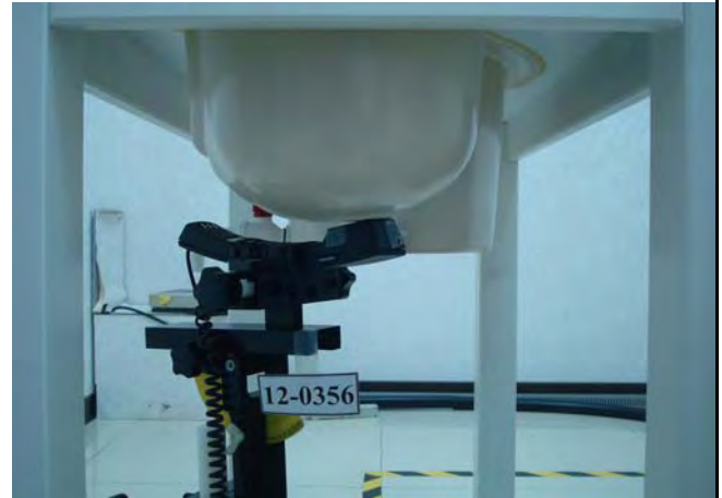
Figure 5. Left Head SAR Test Setup (Tilted)
