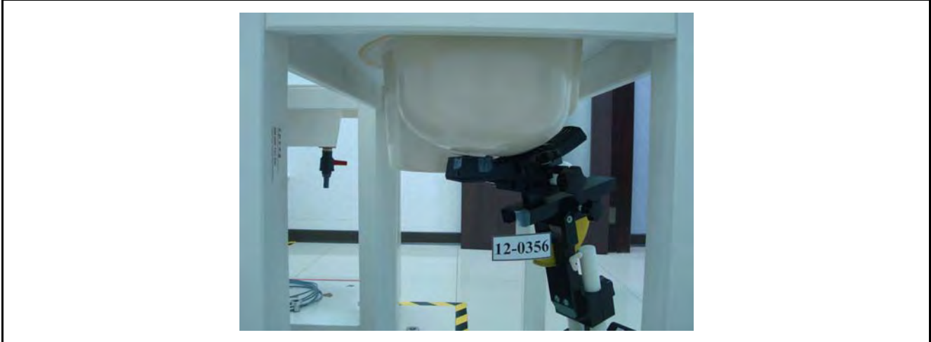
Right Head SAR Test Setup (Cheek)
