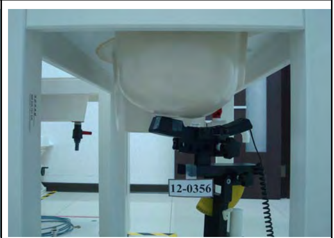
Figure 3. Right Head SAR Test Setup (Tilted)
