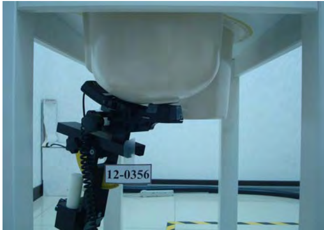
Figure 4. Left Head SAR Test Setup (Cheek)
