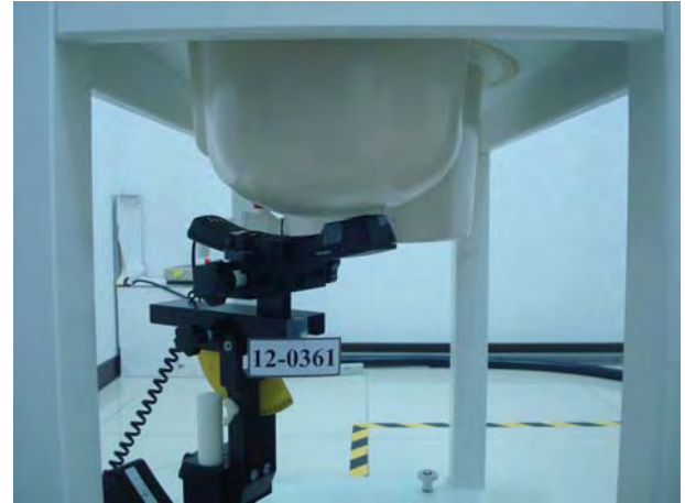
Figure 5. Left Head SAR Test Setup (Tilted)
