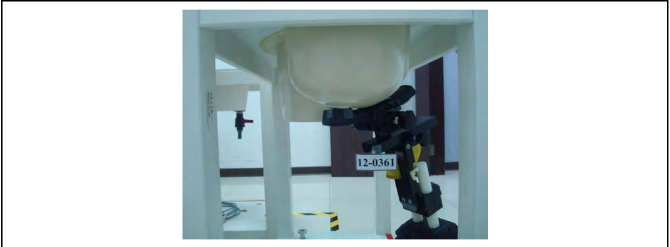
Right Head SAR Test Setup (Cheek)
