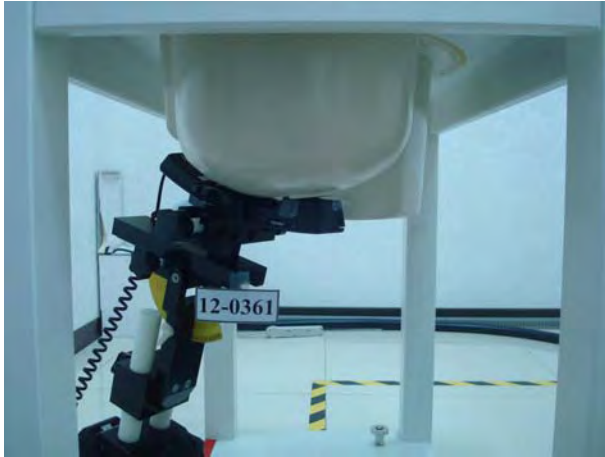
Figure 4. Left Head SAR Test Setup (Cheek)
