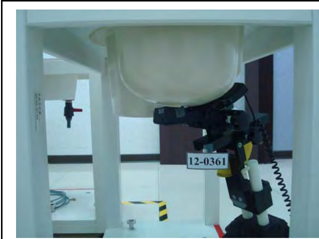
Figure 2. Right Head SAR Test Setup (Cheek)
