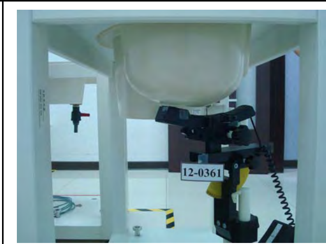
Figure 3. Right Head SAR Test Setup (Tilted)
