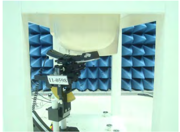
Figure 5. Left Head SAR Test Setup (Tilted)
