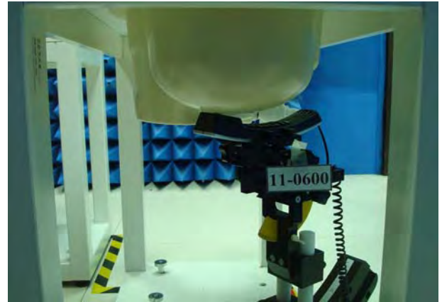
Figure 3. Right Head SAR Test Setup (Tilted)
