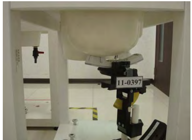
Figure 3. Right Head SAR Test Setup (Tilted)
