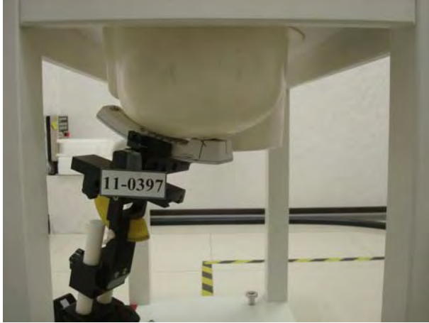
Figure 4. Left Head SAR Test Setup (Cheek)
