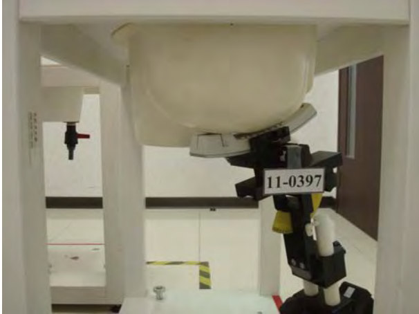
Figure 2. Right Head SAR Test Setup (Cheek)
