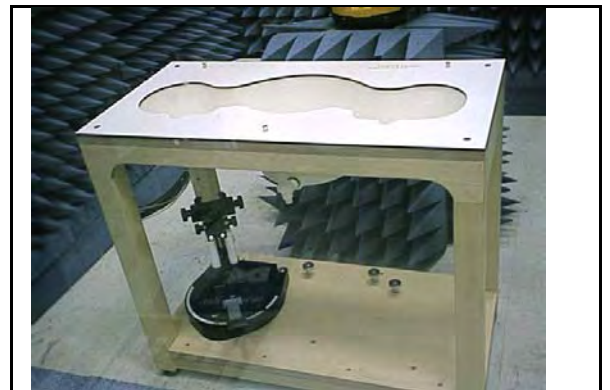
Figure 6. SAM Twin Phantom
