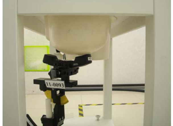
Figure 5. Left Head SAR Test Setup (Tilted)
