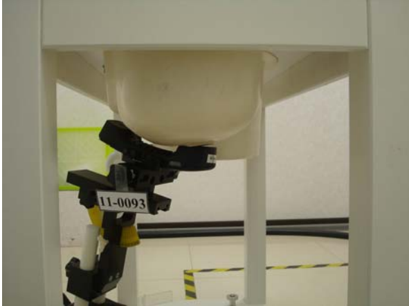
Figure 4. Left Head SAR Test Setup (Cheek)
