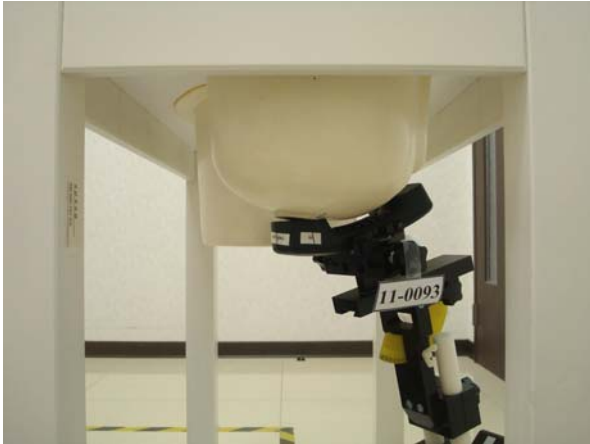
Figure 2. Right Head SAR Test Setup (Cheek)
