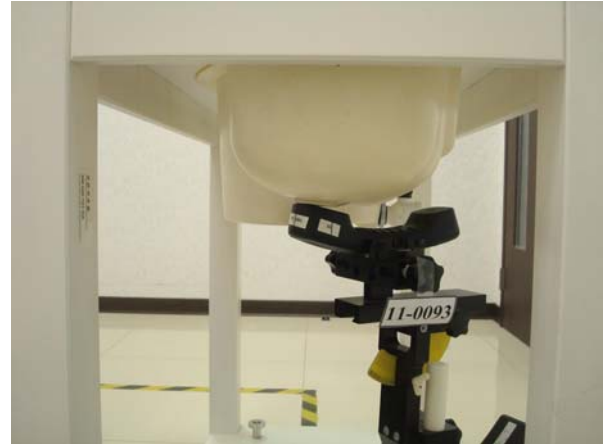
Figure 3. Right Head SAR Test Setup (Tilted)
