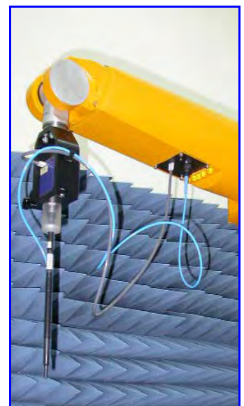
Figure 5. Probe setup on robot
