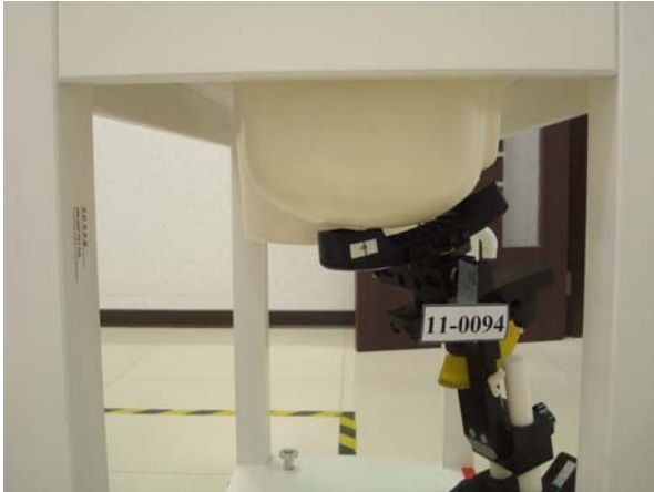
Figure 2. Right Head SAR Test Setup (Cheek)
