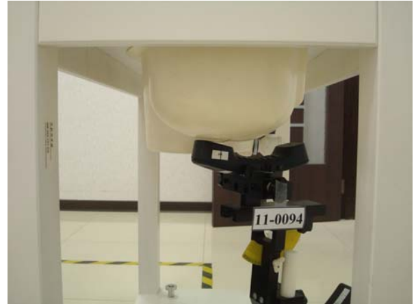
Figure 3. Right Head SAR Test Setup (Tilted)
