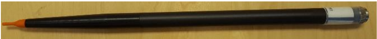
Figure 1 – MVG COMOSAR Dosimetric E field Dipole
