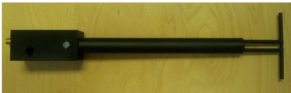
Figure 1 – MVG COMOSAR Validation Dipole
