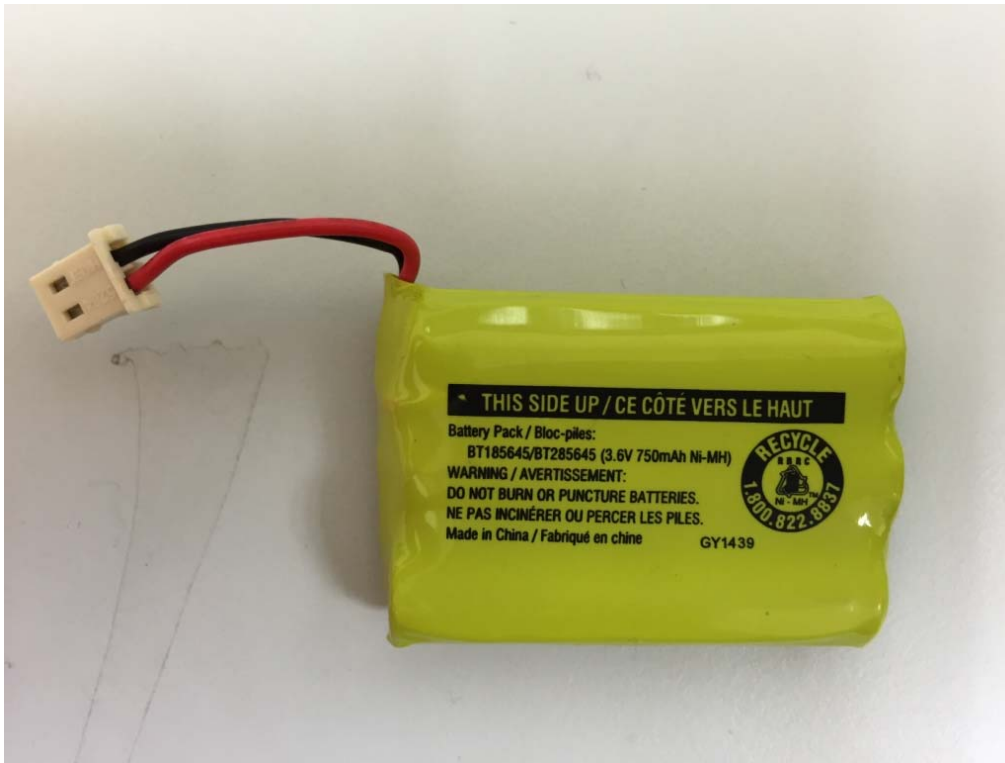
Figure 9 – 3.6V 750mAh Ni-MH Coslight rechargeable battery front view
