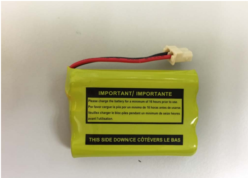
Figure 4 – 3.6V 900mAh Ni-MH GPI rechargeable battery back view
