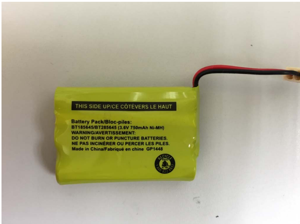
Figure 7 – 3.6V 750mAh Ni-MH GPI rechargeable battery front view
