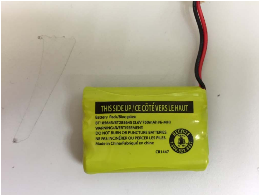
Figure 11 – 3.6V 750mAh Ni-MH Corun rechargeable battery front view
