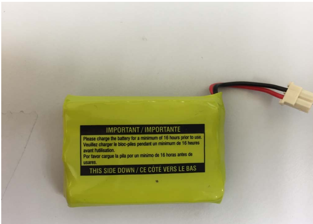
Figure 10 – 3.6V 750mAh Ni-MH Coslight rechargeable battery back view
