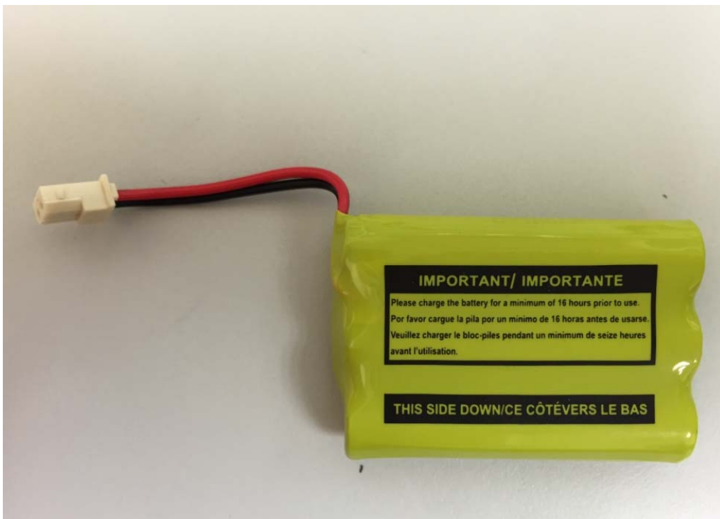
Figure 8 – 3.6V 750mAh Ni-MH GPI rechargeable battery back view
