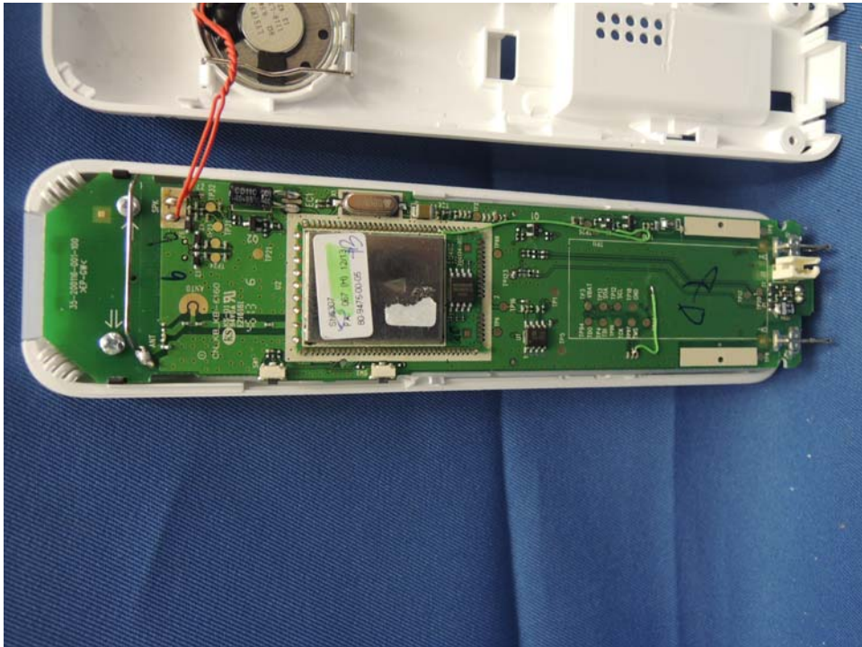
Handset Main PCB comp side (View 1)
