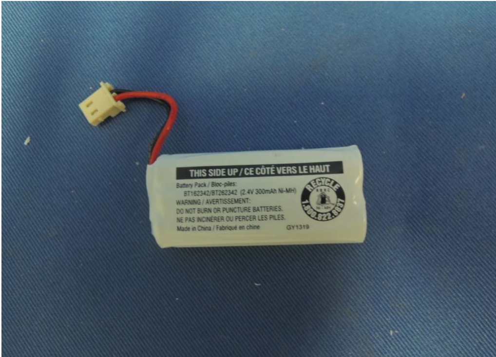
Figure 7 – 2.4VDC 300mAh Coslight battery front view
