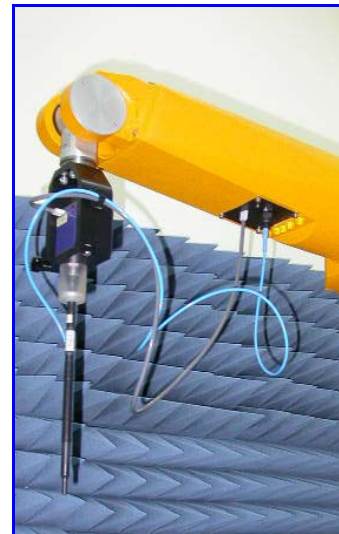
Figure 4. Probe setup on robot
