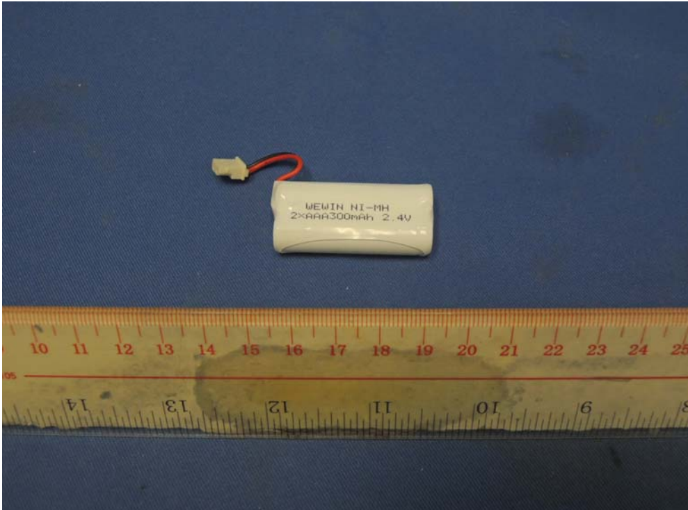
Figure 7 – 2.4VDC 300mAh Wewin rechargeable battery front view
