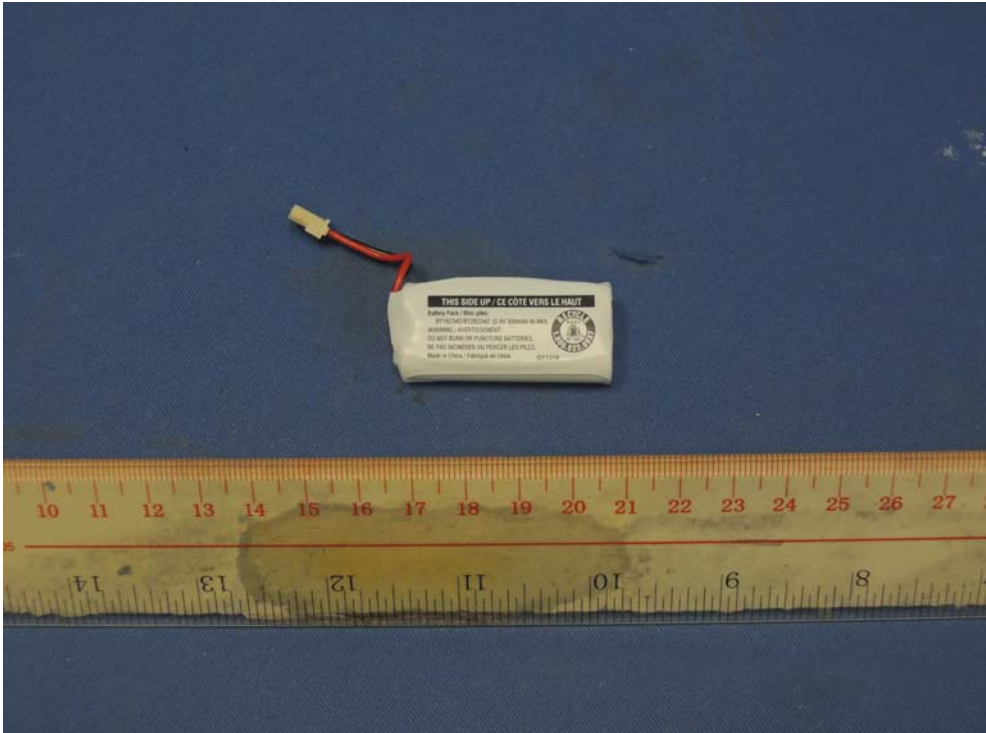
Figure 9 – 2.4VDC 300mAh Coslight rechargeable battery front view
