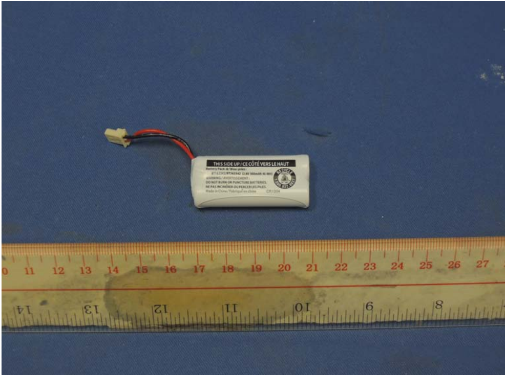
Figure 3 – 2.4VDC 300mAh CORUN rechargeable battery front view
