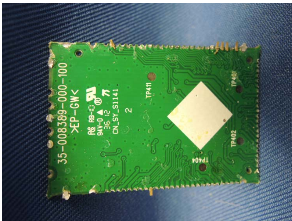
Base Unit Oscillator PCB solder side
