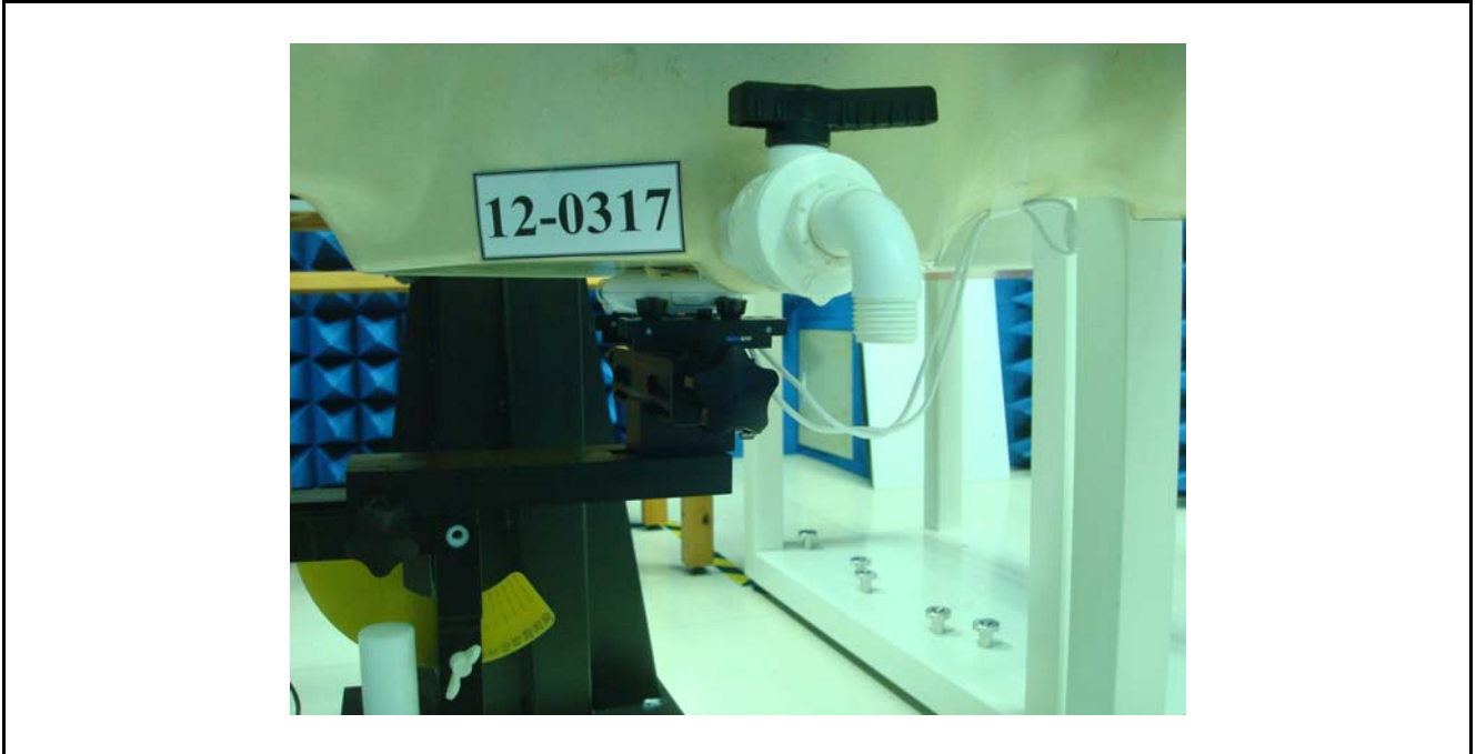
Figure 2. Brain SAR Test Setup (Flat Section)
