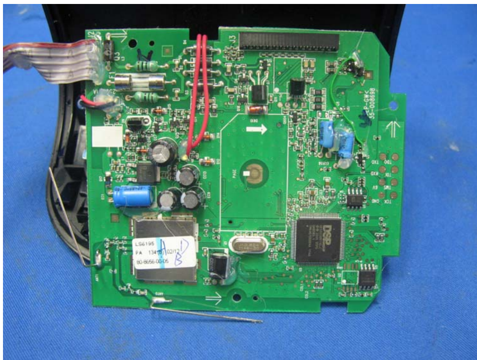
Base Unit Main PCB comp side
