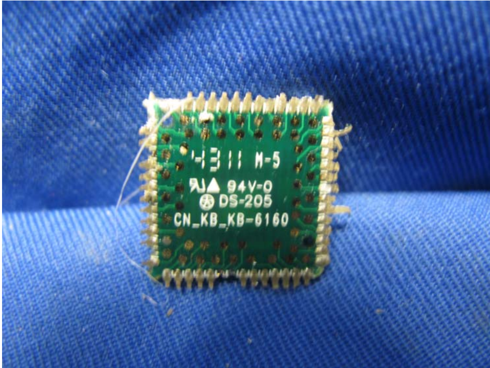
Base Unit Keyboard Controller IC rear side
