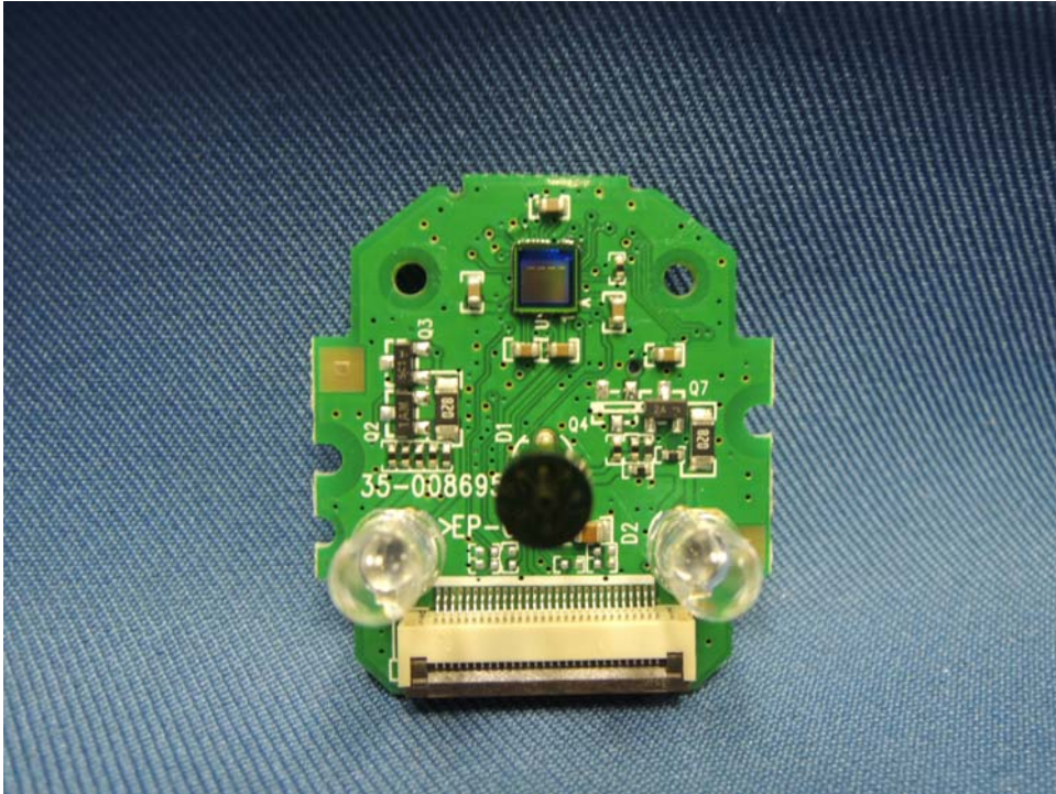
Door Bell Camera Board PCB front side (View 2)
