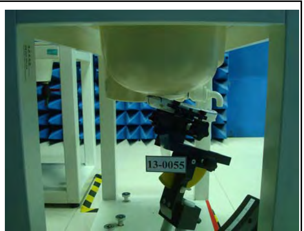
Figure 3. Right Head SAR Test Setup (Tilted)
