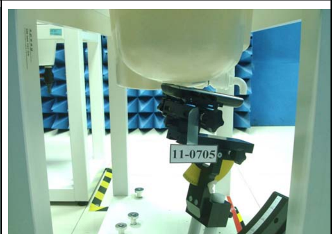
Figure 3. Right Head SAR Test Setup (Tilted)
