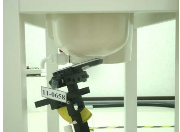
Figure 5. Left Head SAR Test Setup (Tilted)
