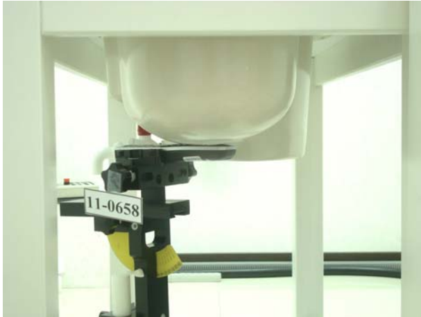
Figure 4. Left Head SAR Test Setup (Cheek)
