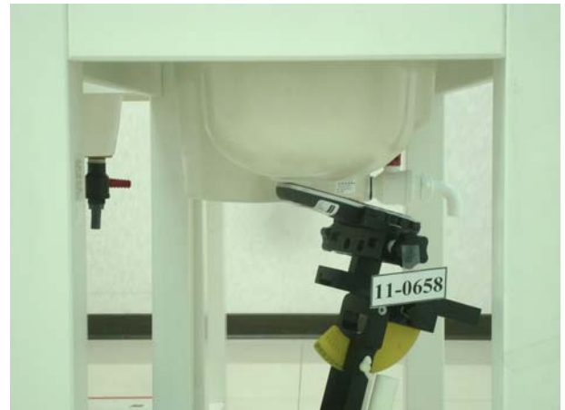
Figure 3. Right Head SAR Test Setup (Tilted)
