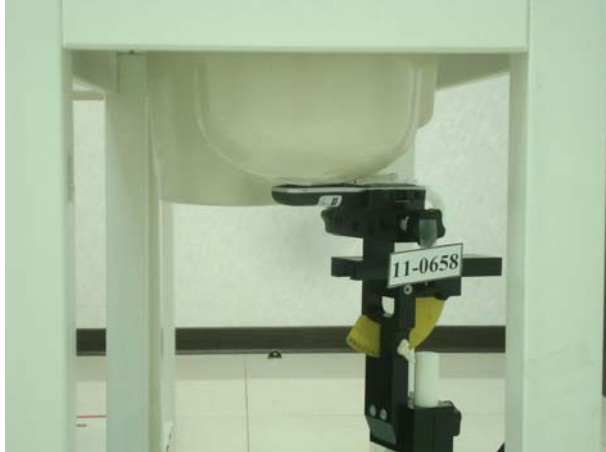
Figure 2. Right Head SAR Test Setup (Cheek)
