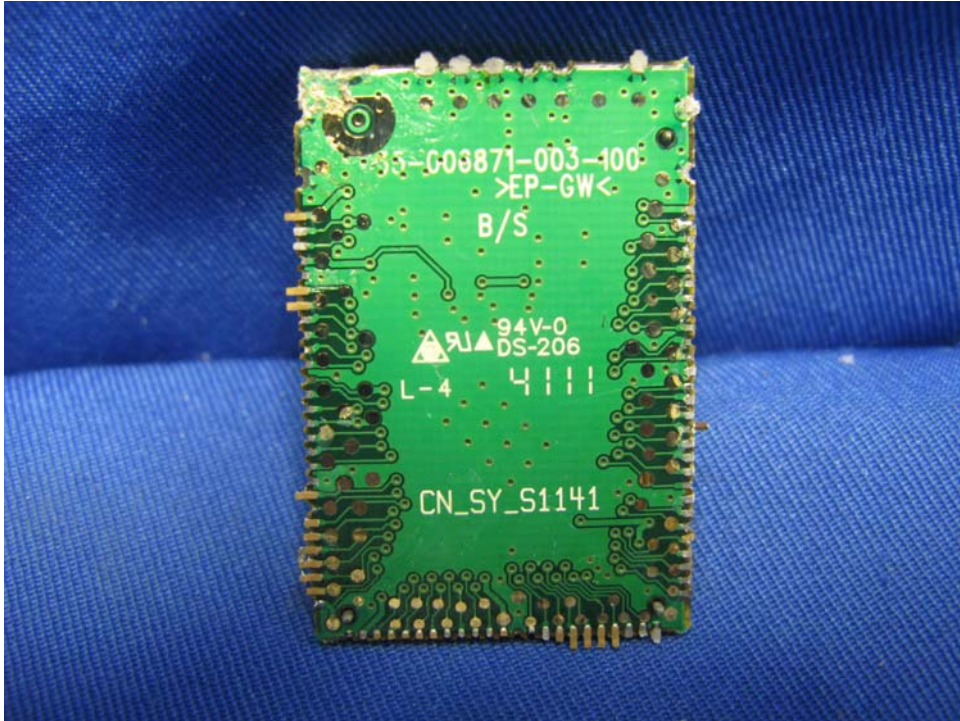
Base Unit Oscillator PCB solder side
