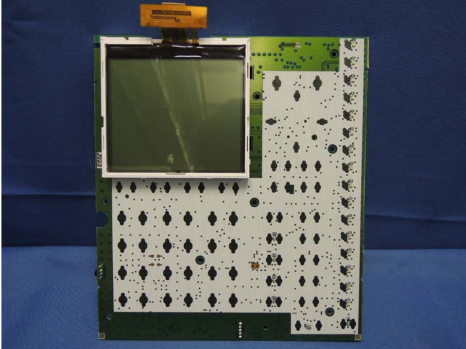
Deskset Keypad and Display front side (View 1)
