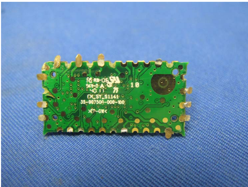
Base Unit Bluetooth RF module solder side
