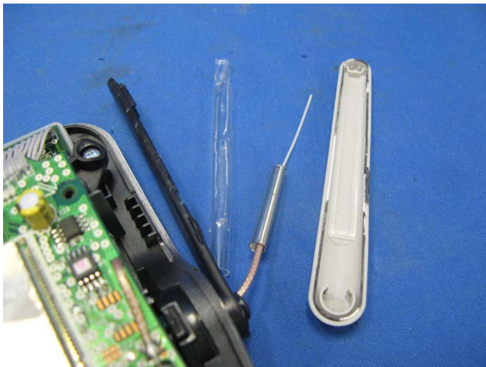
Base Unit DECT antenna
