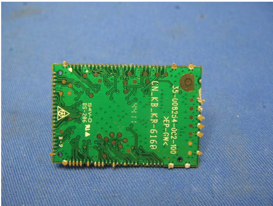
Base Unit DECT RF Module solder side
