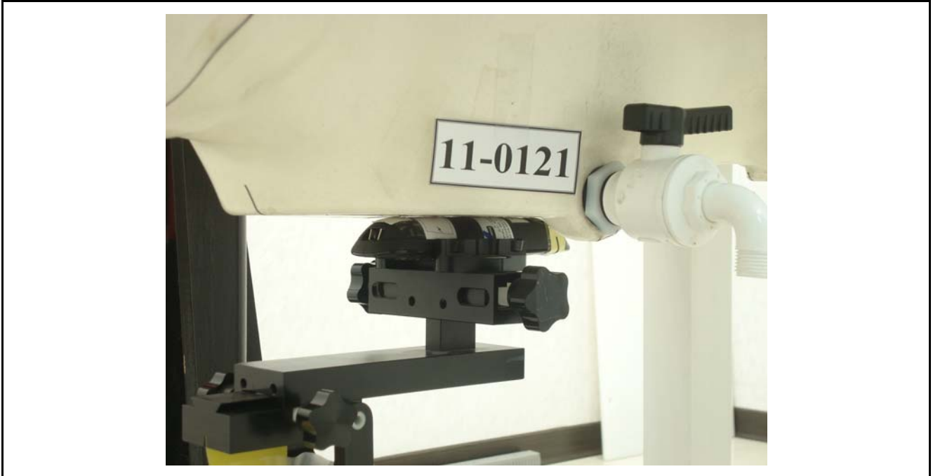
Figure 6. Body SAR Test Setup (Flat Section)
