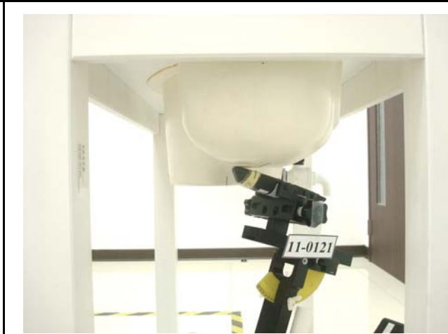
Figure 3. Right Head SAR Test Setup (Tilted)
