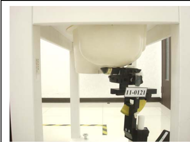
Figure 2. Right Head SAR Test Setup (Cheek)
