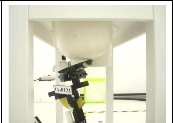
Figure 5. Left Head SAR Test Setup (Tilted)
