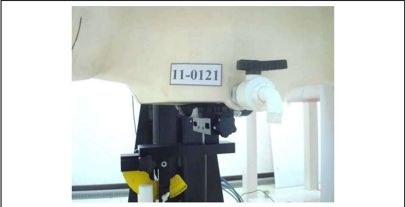
Figure 7. Body SAR Test Setup (Flat Section)
