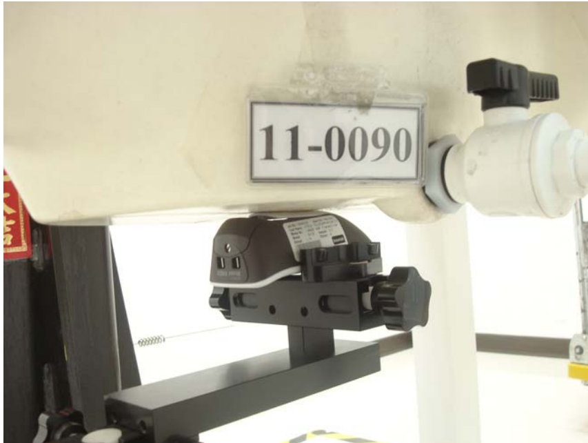
Figure 2. Body SAR Test Setup (Flat Section)
