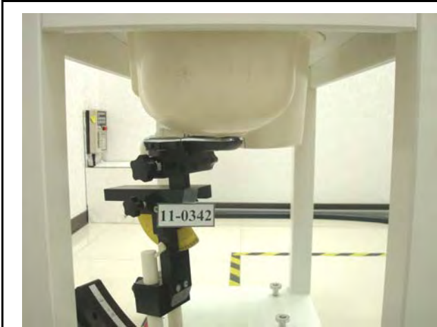
Figure 4. Left Head SAR Test Setup (Cheek)
