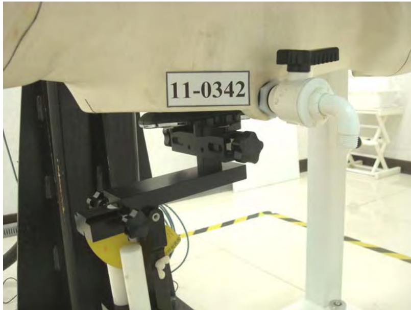
Figure 7. Body SAR Test Setup (Flat Section)
