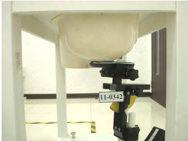
Figure 2. Right Head SAR Test Setup (Cheek)
