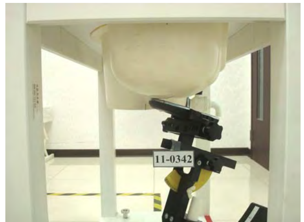
Figure 3. Right Head SAR Test Setup (Tilted)
