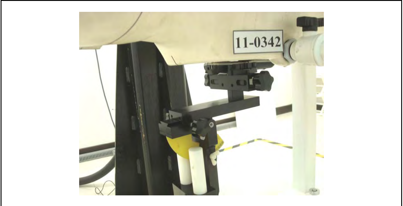
Figure 6. Body SAR Test Setup (Flat Section)
