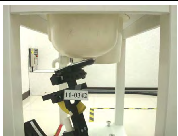
Figure 5. Left Head SAR Test Setup (Tilted)
