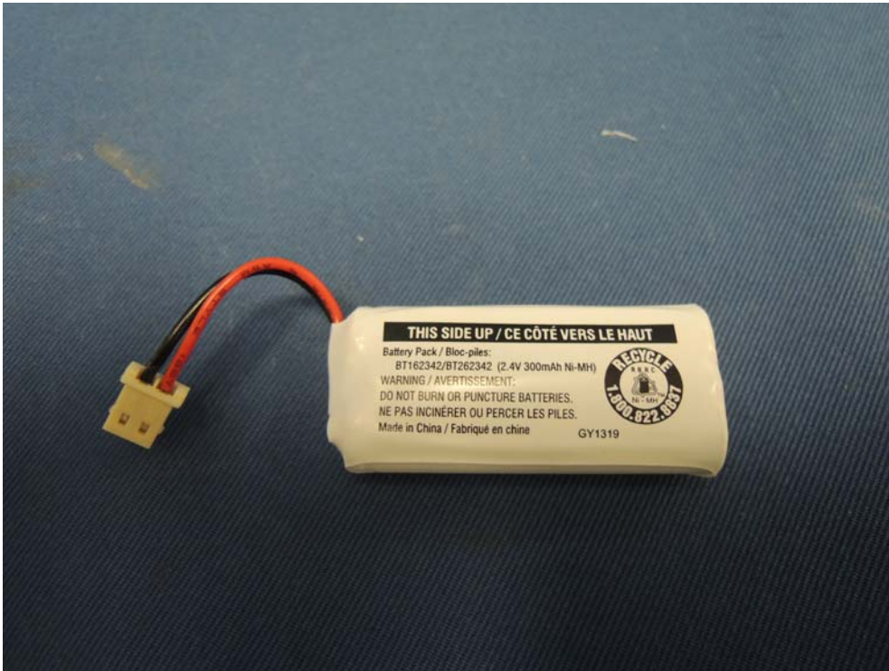
Figure 5 – 2.4V 300mAh Ni-MH Coslight rechargeable battery front view
