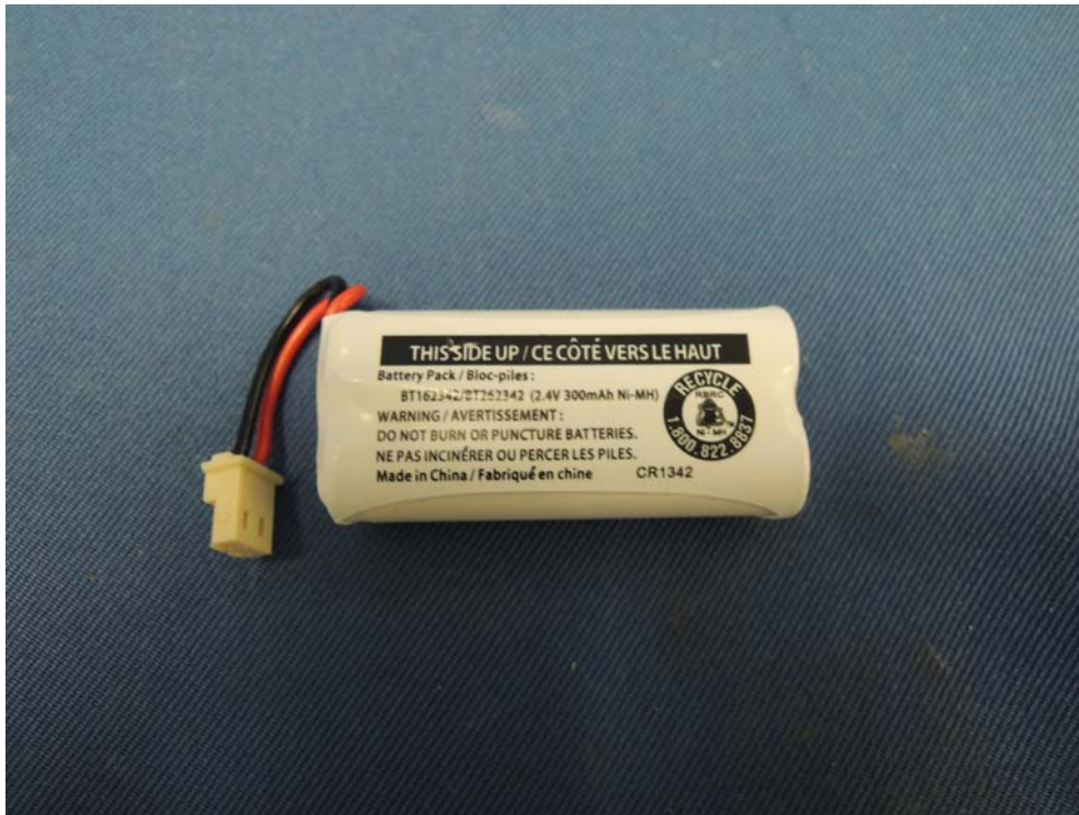
Figure 3 – 2.4V 300mAh Ni-MH Courn rechargeable battery front view
