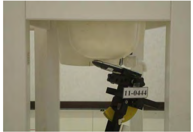
Figure 3. Right Head SAR Test Setup (Tilted)
