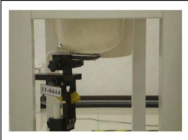
Figure 4. Left Head SAR Test Setup (Cheek)
