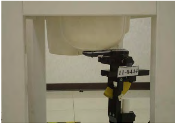
Figure 2. Right Head SAR Test Setup (Cheek)
