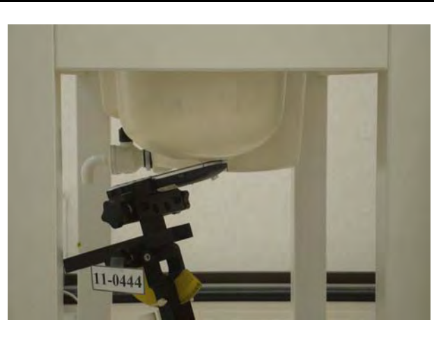
Figure 5. Left Head SAR Test Setup (Tilted)
