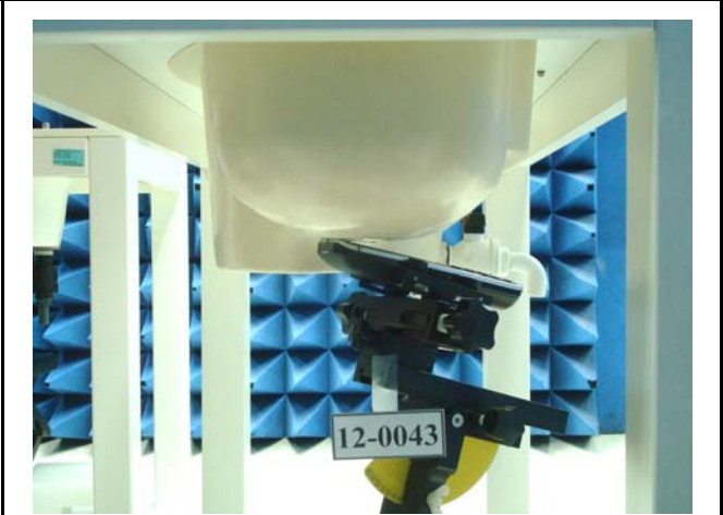
Figure 3. Right Head SAR Test Setup (Tilted)
