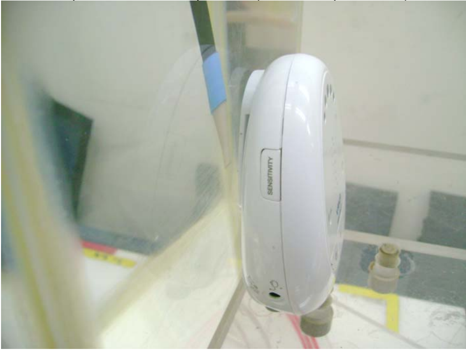
EUT rear to phantom, 0 mm separation (with belt clip mounted)– Zoom In
