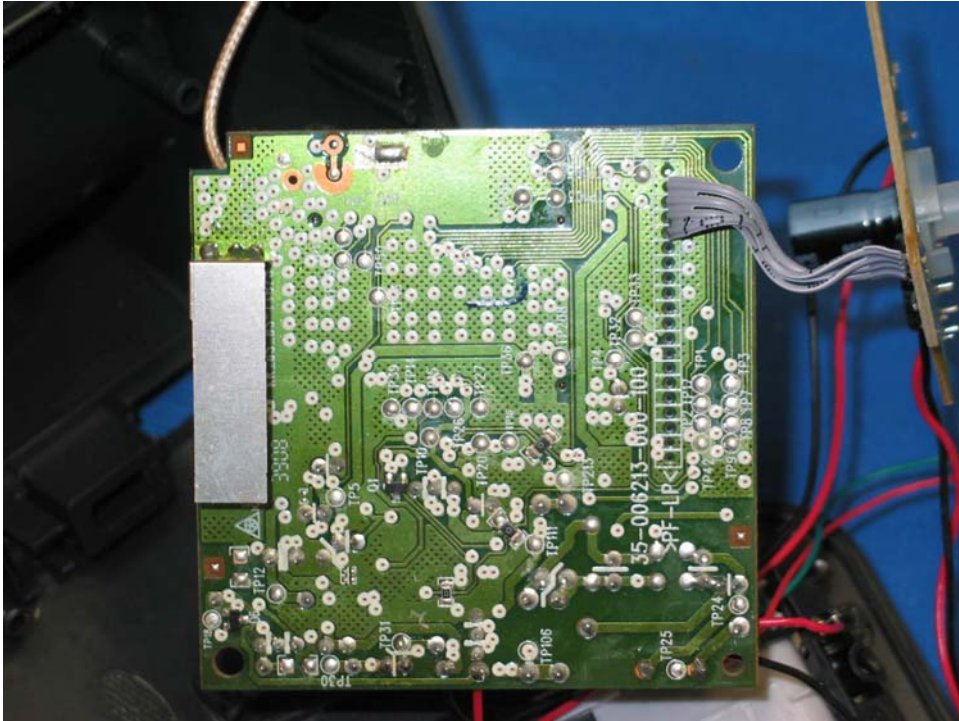
Base Unit Main PCB solder side
