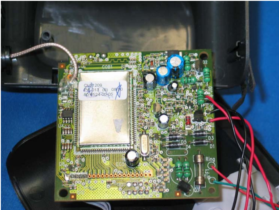
Base Unit Main PCB comp side
