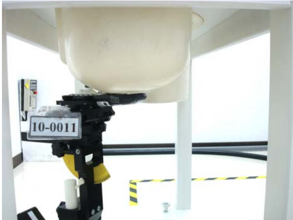
Figure 4. Left Head SAR Test Setup (Cheek)
