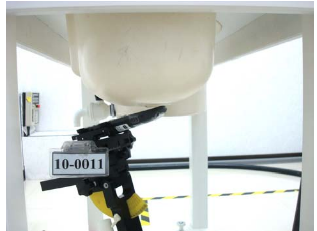
Figure 5. Left Head SAR Test Setup (Tilted)
