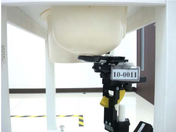
Figure 2. Right Head SAR Test Setup (Cheek)
