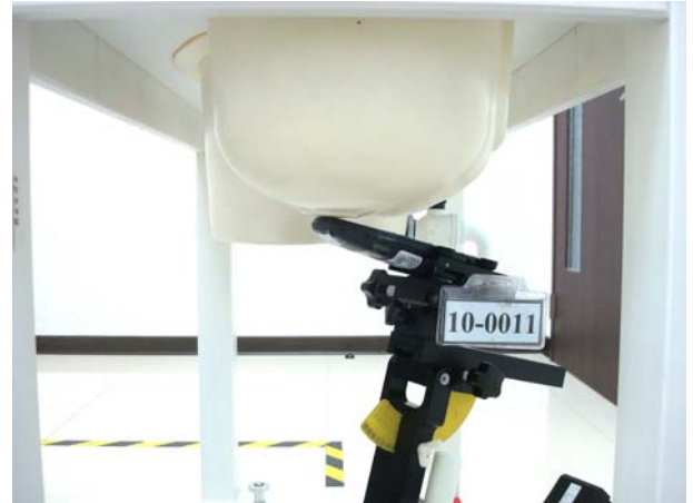
Figure 3. Right Head SAR Test Setup (Tilted)
